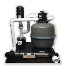
Step 2: Set the filter, pump and UV on the pad as shown. Place media Agitator on Check valve. Do not glue Agitator to pipe. Use a set screw through the pipe and agitator throat if needed to hold it. Connect like number to like number by tightening the unions together by hand.
