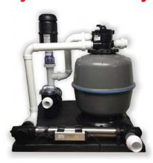
Step 3: Attach the ZapTek UV to the filter outlet as shown. Attach pipe to pump and inlet of filter. Hand tighten only the unions. Make sure the gaskets are in the unions at the connections.
